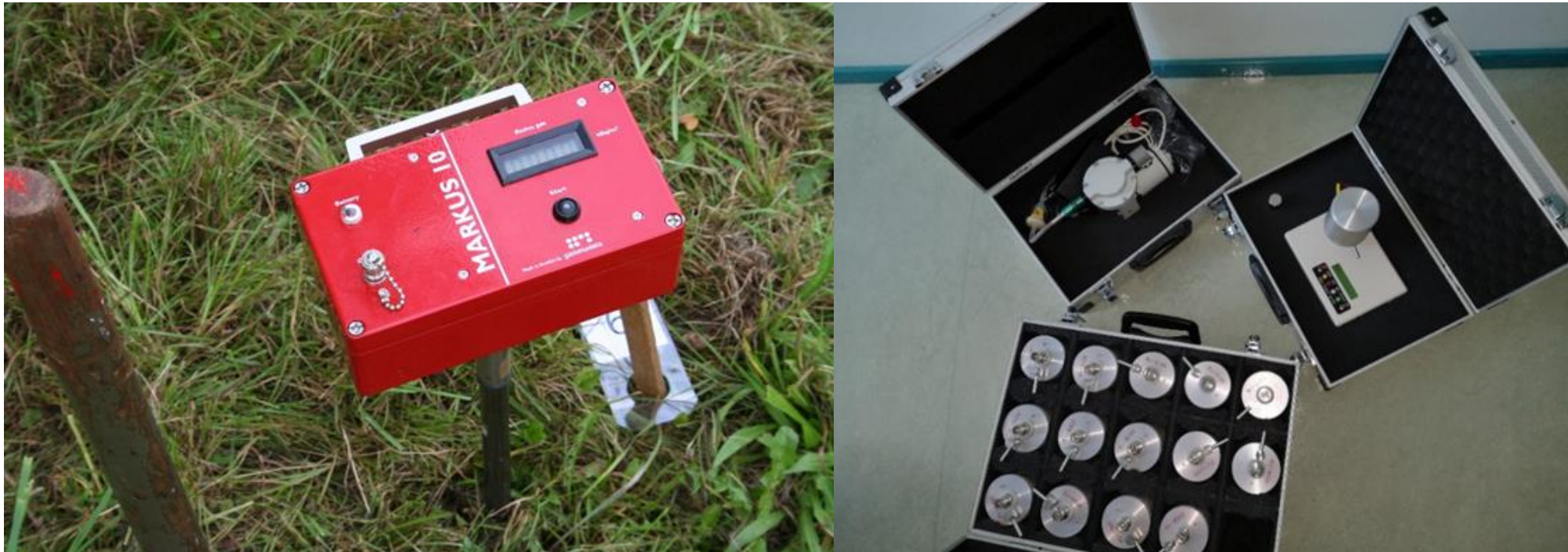
Photo 1. Emanometer Markus 10 on the left and RM-2 on the right for measuring radon directly from soil air
