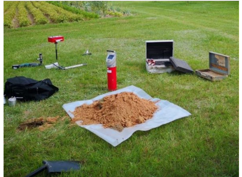
Photo 2. Measuring radon indirectly with spectrometer
